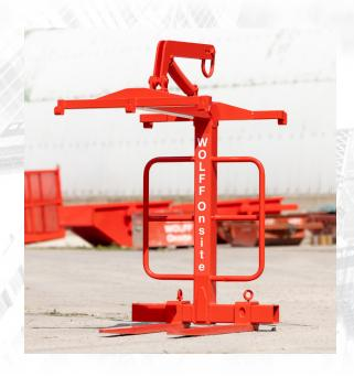
Self levelling brick forks are designed to lift brick packs and pallets, by using the adjustable forks.
