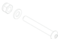
4x M10 Button Head Screw, M10 Washer and M10 Nylock Nut
